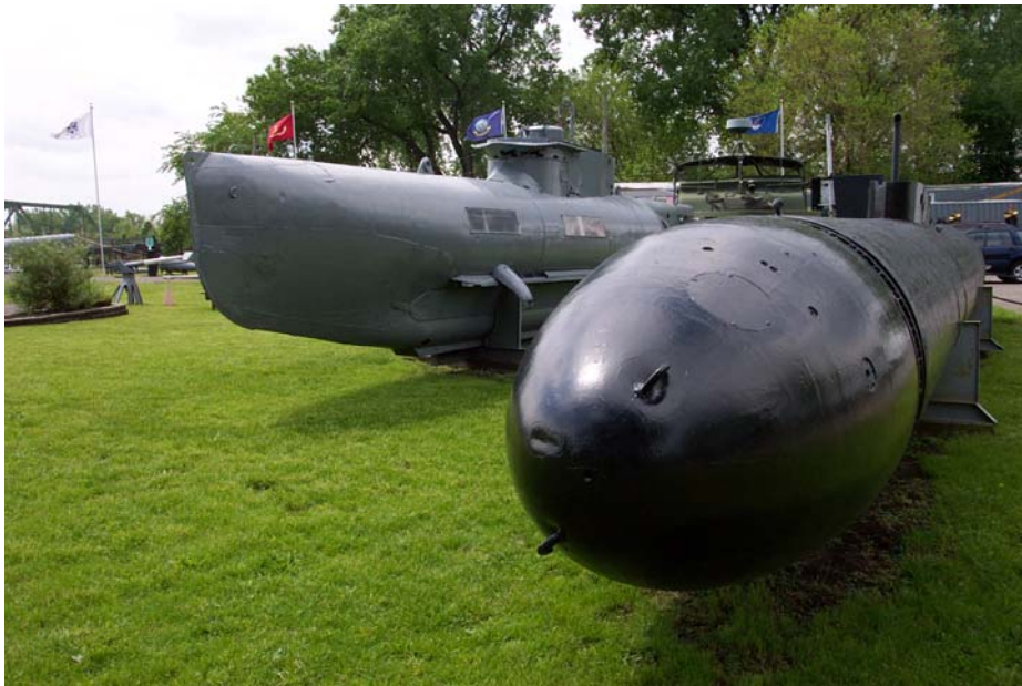
NJ Naval Museum is home to other important wart relics, such as this Japanese Kaiten II torpedo pictured in the foreground. It was a 2-man human torpedo filled with 3,417 lbs of explosives; it was used to sink US ships during WW2.
