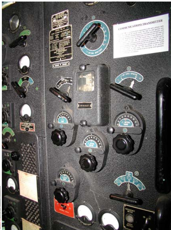
US Navy TLB-12 Transmitter capable of 200 watts on CW.
